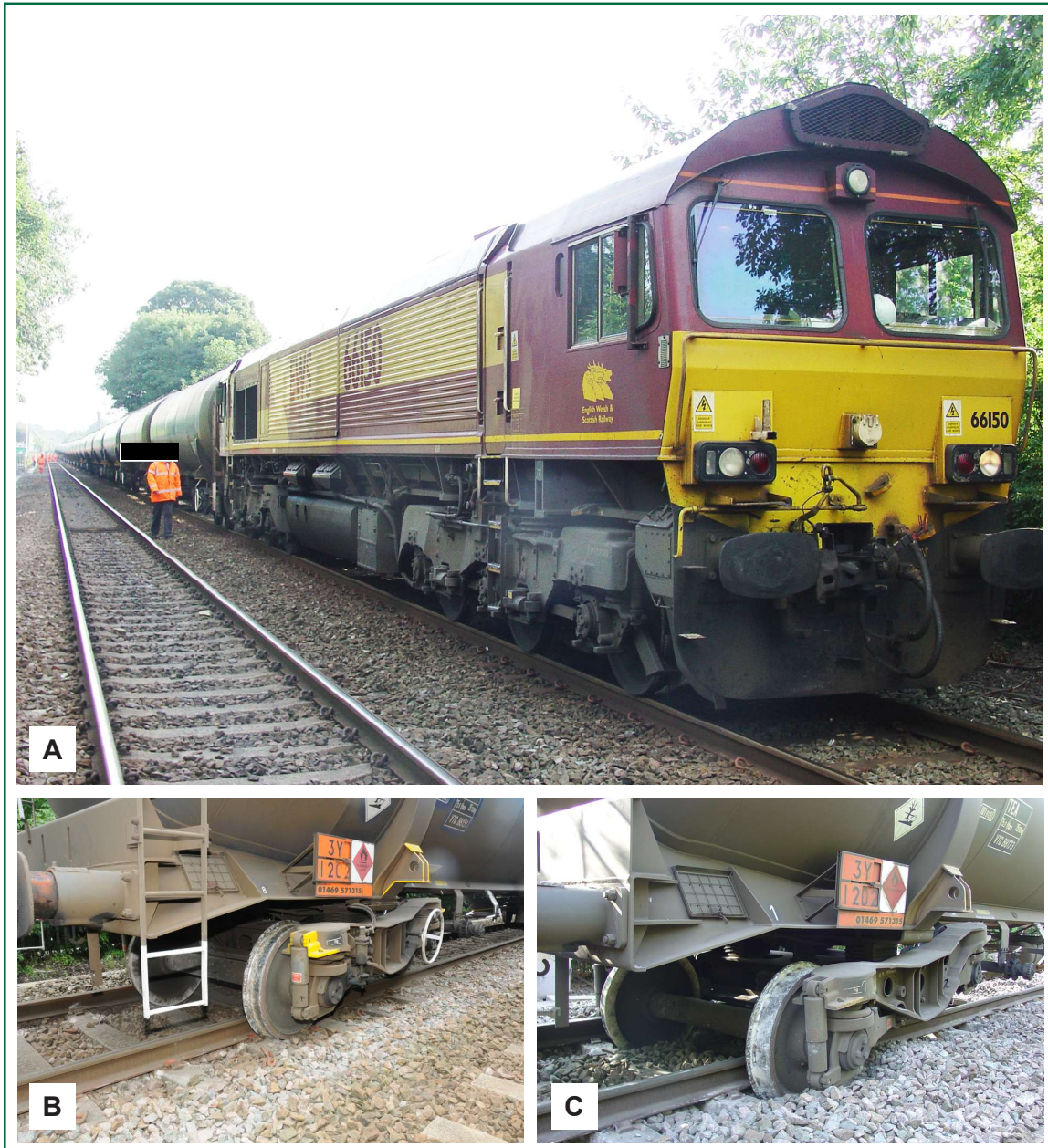
Figure 2: Train 6M35 (a) and its derailed wheelsets on 26th wagon (b) and 28th wagon (c)
